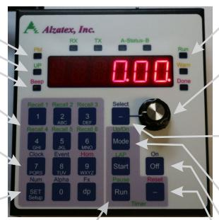
Momentarily press **Run** or **Start** to start the timer, press Run again to stop it or press Start again to pause the display for a short time but continue running the timer internally (Lap Mode).
