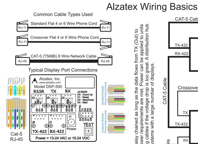
The TX, RX, TX-422 and RX-422 ports are for serial data connections between Timers and Displays. The TX and RX ports are RJ-11 type and use 4 wire phone cords. They are used for short distance connections (<100ft). The TX-422 and RX-422 ports are RJ-45 type and use 8 wire CAT-5 network cable. They are used for longer distance connections. TX (Out) connects to RX (In) or TX-422 (Out) connects to RX-422 (In).
