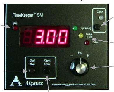
Real Time Clock. Press to show the time in 24H or 12H mode. Press and Hold to set the current time (Hour then Minute then Second, using the knob to change the value and pressing the Clock button to move to the next value).
